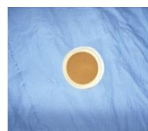
The **QSA** test allows to differentiate the soft contaminants, (the latter being responsible for the formation of varnish) from the hard and larger contaminants (not being related to oil degradation).
